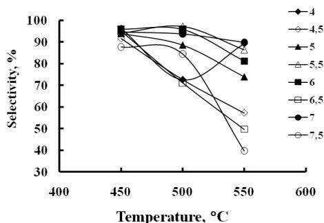
Fig. 4. Effect of temperature on the selectivity by the light petroleum products of the catalytic cracking process in the aerosol catalyst of type Y at oscillation frequency of the reactor from 4 to 7,5 Hz
