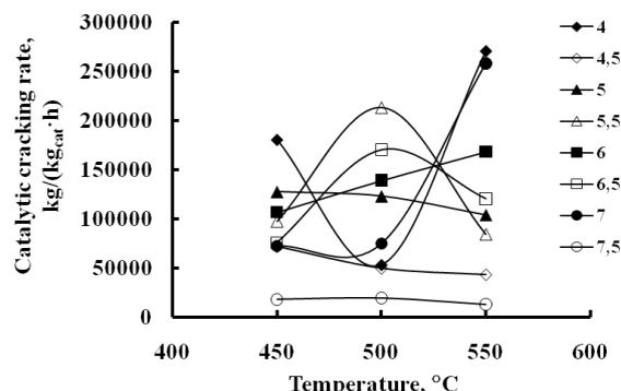
Fig. 5. Effect of temperature on the catalytic cracking rate by the mass of aerosol catalyst of type Y at oscillation frequency of the reactor from 4 to 7,5 Hz
