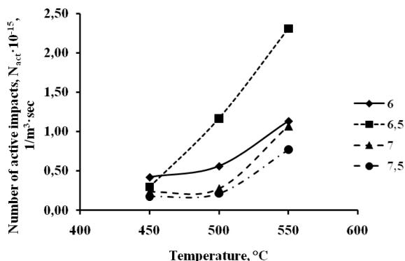
Fig. 7. Effect of temperature on the number of active impacts of particles of the catalyst of type Y at oscillation frequency of the reactor from 6 to 7.5 Hz
