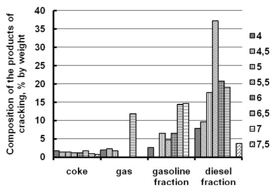
Fig. 2. Composition of products of the catalytic cracking reaction in the aerosol catalyst of type Y at temperature 500 °C and different reaction oscillation frequency
