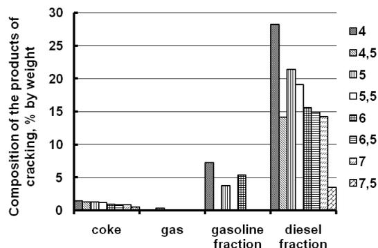
Fig. 1. Composition of products of the catalytic cracking reaction in the aerosol catalyst of type Y at temperature 450 °C and different reaction oscillation frequency
