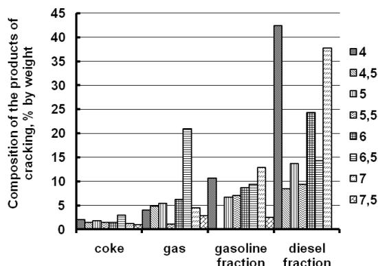
Fig. 3. Composition of products of the catalytic cracking reaction in the aerosol catalyst of type Y at temperature 550 °C and different reaction oscillation frequency
