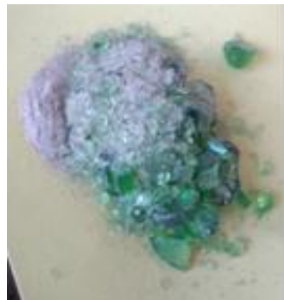
Figure 4. Preparation and grinding fraction of glass
