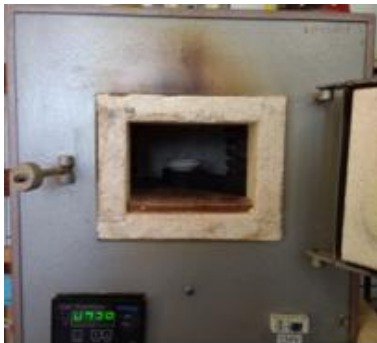
Figure 1. The muffle furnace when the operating mode is reached and inside with the capacity of the studied mixture of substances as a heat carrier
